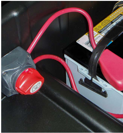
BATTERY SHUT OFF SWITCH 850-242
