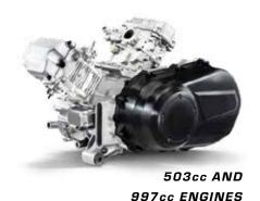
**Engines** – The 503cc single cylinder and the 997cc twin cylinder 4-stroke engines feature electronic fuel injection (EFI), single overhead cam and liquid cooling with an auxiliary fan that provides consistent performance in the most demanding conditions. Both engines are clean and deliver class-leading horsepower and incredible torque.
