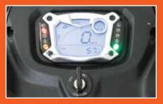
**INSTRUMENT GAUGE**Digital display features odometer, speedometer, trip odometer, RPM, EPS setting and fuel level. Surrounding the display are easy-to-identify indicators for transmission position, high temp, low battery, high beam, low oil pressure, check engine, 2wd/4wd and differential lock indicators.
