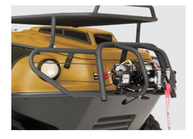
ARGO's 3,500 lb. (1,588 kg) winch mounts front or back to assist with self recovery.
