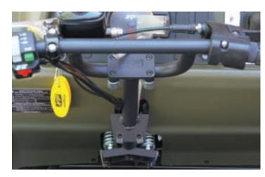
By adding a spring element between the handlebars and the brake system, we achieved a progressive dual-rate steering system.
