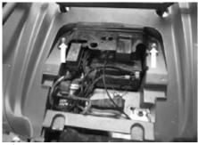
4. Remove the battery from the compartment.
