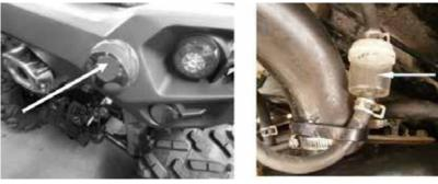
There is a sight glass located near the fuel fill to check the over full tank during refilling.
