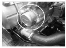
11. Refill with the specified amount of the recommended engine oil (10W40). Install and tighten the engine oil filler cap.
