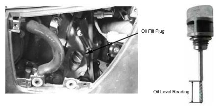
Insert the dipstick into the filler hole (by screwing it in) and then remove it again to check the oil level.
