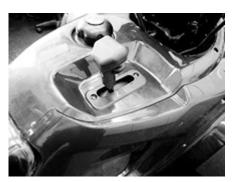
Note: When shifting from H to L and any gear/direction, the vehicle must be at a complete stop.
