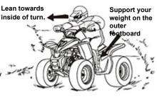
As you approach a curve, slow down and begin to turn the handlebars in the desired direction. As you do so, put your weight on the footboard to the outside of the turn (opposite your desired direction) and lean your upper body into the turn. Use the throttle to maintain an even speed through the turn. This maneuver will let the wheel on the inside of the turn slip slightly, allowing the ATV to make the turn properly.
