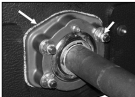
Re-tightening nuts (mid axles).
