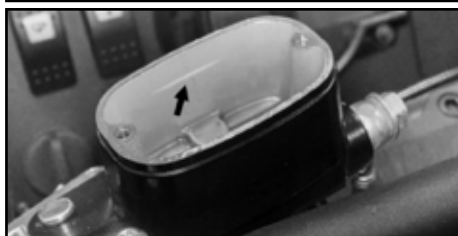
Hydraulic brake cylinder and fluid level.
