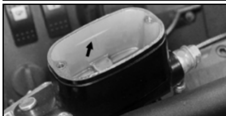
Hydraulic brake cylinder and fluid level.
