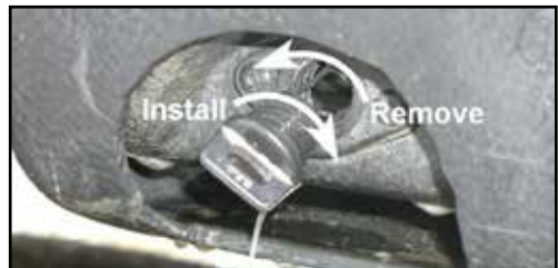
Location of rear drain plugs.
