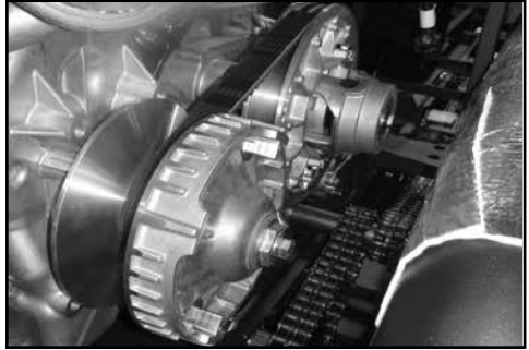
Location of drive clutches and drive belt.
