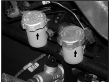
Hydraulic brake cylinder and fluid level.
