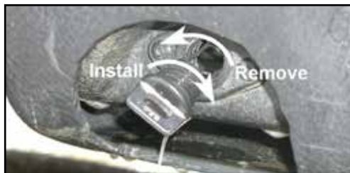
Location of rear drain plugs.
