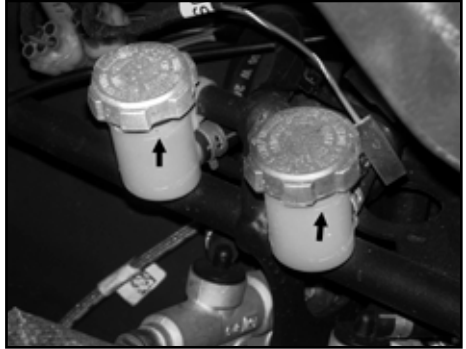
Hydraulic brake cylinder and fluid level.
