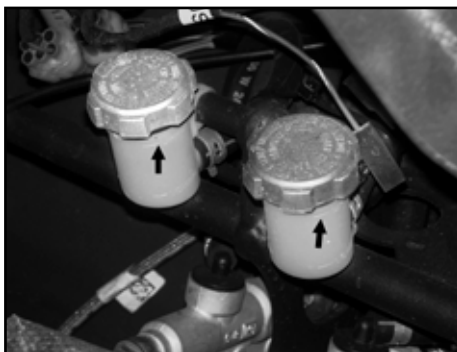
Hydraulic brake cylinder and fluid level.
