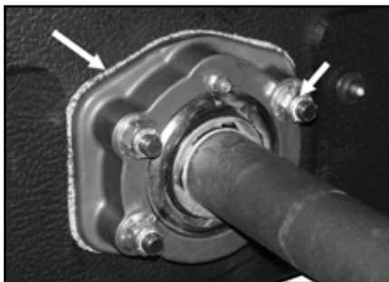
Re-tightening nuts (mid axles).
