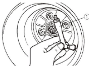
Low-pressure tire gauge
