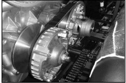
Location of drive clutches and drive belt.
