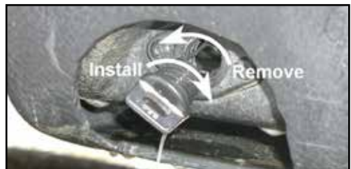
Location of rear drain plugs.
