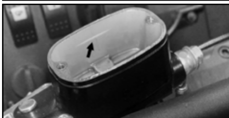
Hydraulic brake cylinder and fluid level.
