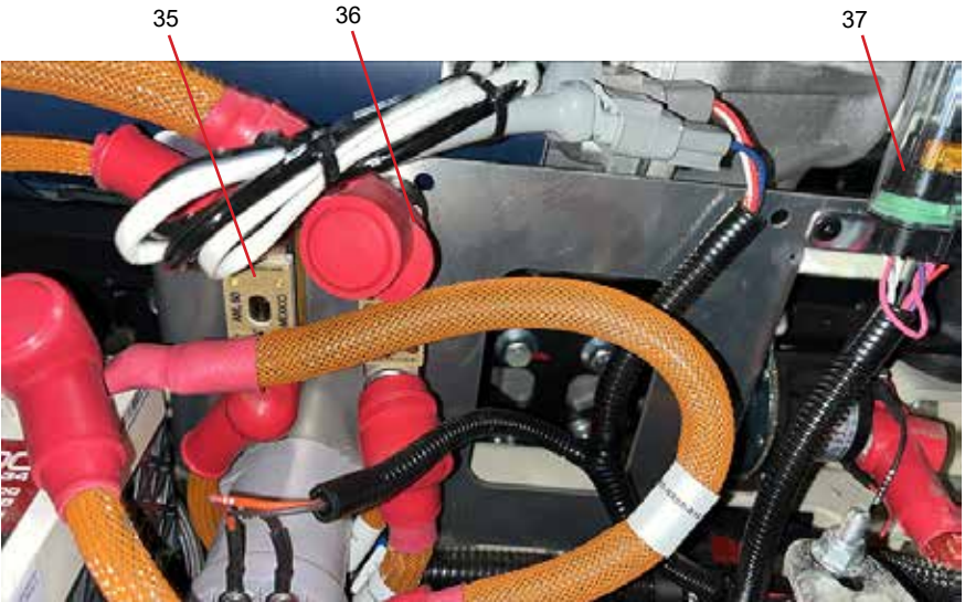
35. Fan Power Fuse Block 37. Steering Relay
