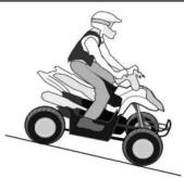
Avoid sudden application of either the front or rear brake because the wheels on the uphill side could come off the ground.
