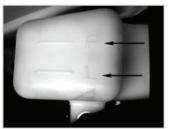
If the coolant is at or below the minimum level mark, remove the coolant reservoir cap, add coolant or distilled water to the maximum level mark and install the reservoir cap.
