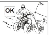
If you must cross the side of a hill or turn on a hill: Always follow proper procedures described in this Operator's Manual. Avoid hills with slippery or loose surfaces.
