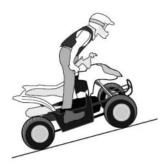
Do not attempt to climb hills until you have mastered basic maneuvers on flat ground. Always check the terrain carefully before attempting any hill. In all cases avoid inclines with slippery or loose surfaces or obstacles that might cause you to lose control.
