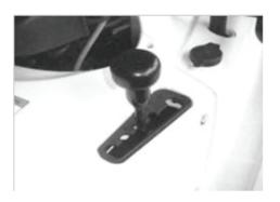
Note: When shifting from H to L and any gear/direction, the vehicle must be at a complete stop.
