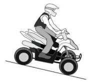
Avoid sudden application of either the front or rear brake because the wheels on the uphill side could come off the ground.
