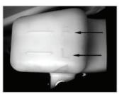
If the coolant is at or below the minimum level mark, remove the coolant reservoir cap, add coolant or distilled water to the maximum level mark and install the reservoir cap.
