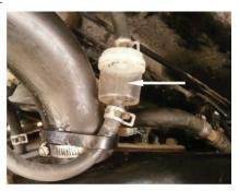
There is a sight glass located near the fuel fill to check the over full tank during refilling.
