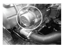
11. Refill with the specified amount of the recommended engine oil (10W40). Install and tighten the engine oil filler cap.
