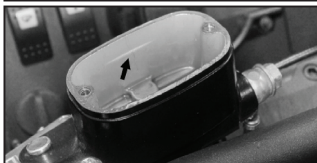
Hydraulic brake cylinder and fluid level.
