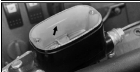
Hydraulic brake cylinder and fluid level.
