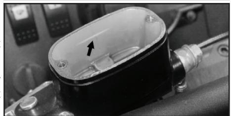
Hydraulic brake cylinder and fluid level.
