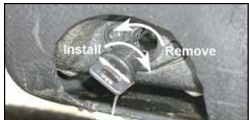
Location of rear drain plugs.
