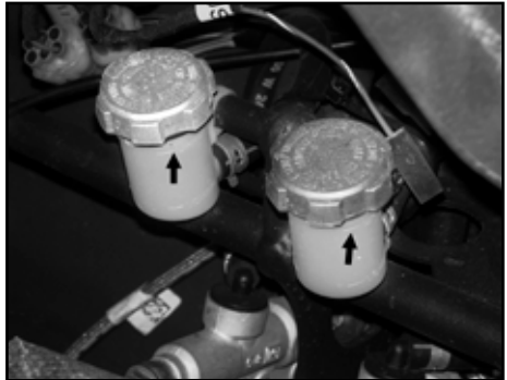
Hydraulic brake cylinder and fluid level.
