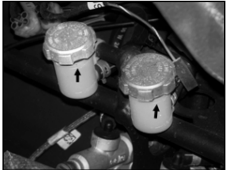
Hydraulic brake cylinder and fluid level.
