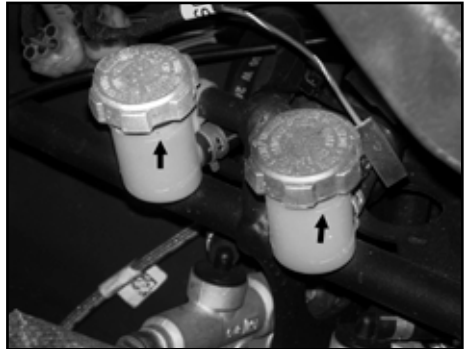
Hydraulic brake cylinder and fluid level.
