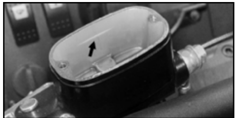
Hydraulic brake cylinder and fluid level.
