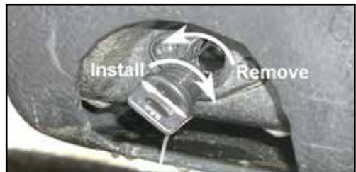
Location of rear drain plugs.
