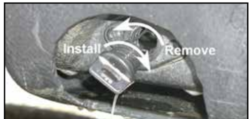
Location of rear drain plugs.
