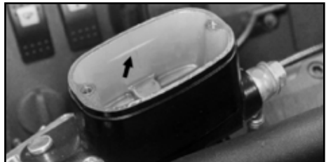
Hydraulic brake cylinder and fluid level.
