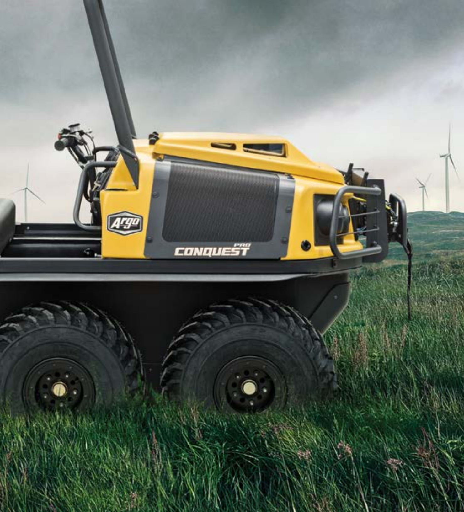
25" XT119 Tires on AirLock™ Steel Rims
